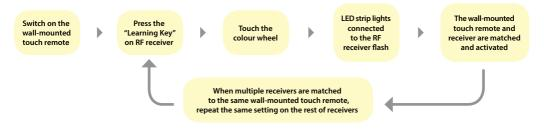
Alternative way to match RF receiver when it is difficult to reach the receivers.
