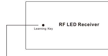
**Step 2:** Short press the "Learning Key" button on RF receiver or re-power on the receiver three times continuously to set it into pairing status
